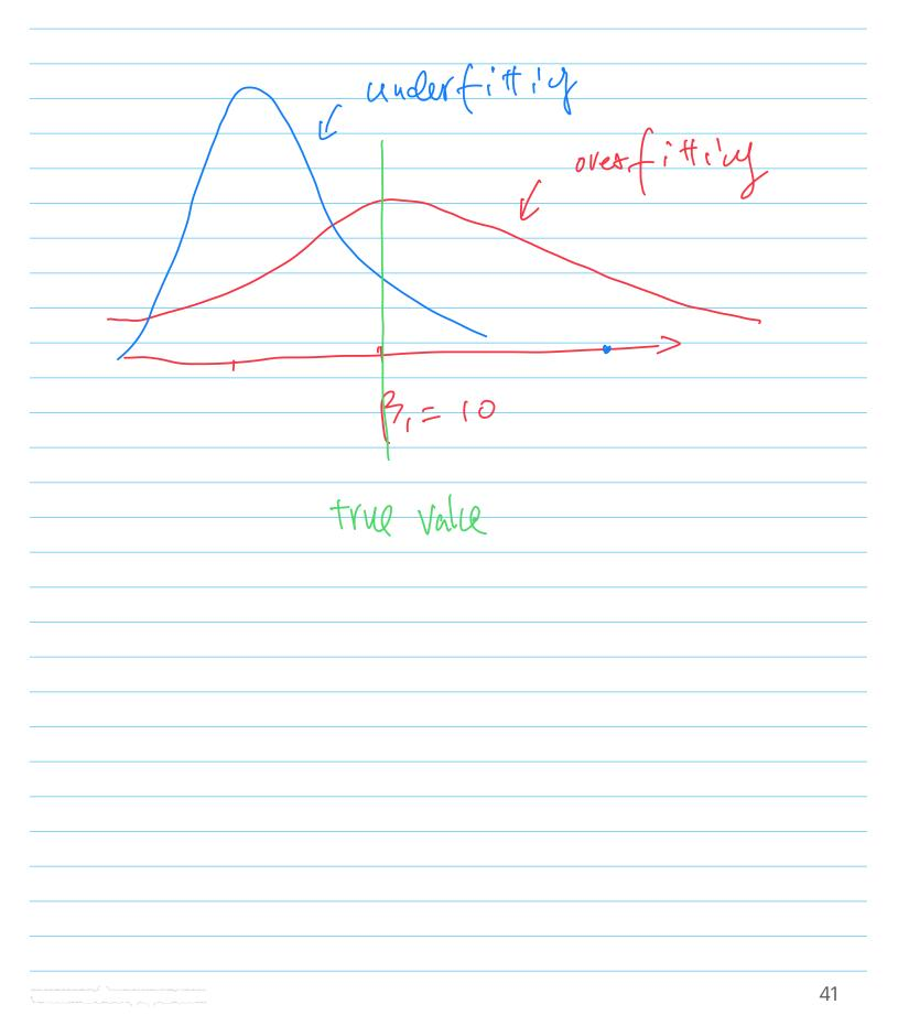
To summarize, we've seen that underfitting reduces the variances of regression parameter estimators, but introduces bias. On the other hand, overfitting produces unbiased estimators with increased variances. Thus it is the task of a regression model builder to find an optimum set of explanatory variables to balance between a biased model and one with large variances.
